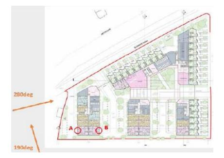
218. The image below shows the location of the balconies within the site (highlighted in blue). There are certain balconies (highlighted red), which are exposed to the onset wind. However these balconies are proposed to have glass balustrades, which will provide mitigation against this.
